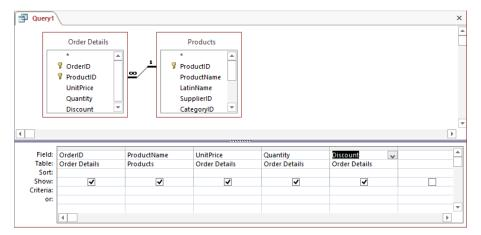
The results datasheet will display the extracted information in the order of the fields in the design grid.
