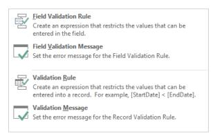
The top set of options is for validating the field and the bottom set is for validating the entire record.
