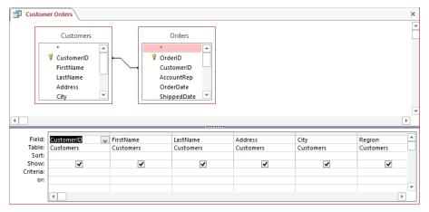
The top pane identifies the tables used by the query and the relationship between them. In the design grid, the Field row identifies the fields used, the Table row identifies each field's table, and selected check boxes in the Show row indicate the fields to display in the results.
