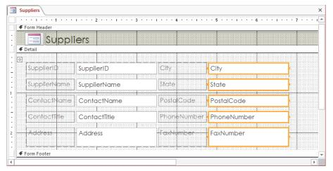
In Design View, Access displays horizontal and vertical rulers and a grid to help you position controls and labels.
