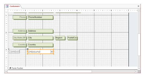
Because the combo box control is not attached to a field in the Customers table, its name is Unbound.
