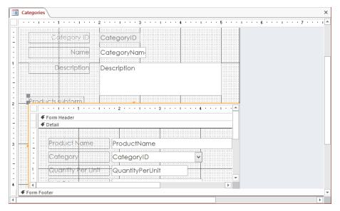
The subform control has its own Form Header, Detail, and Form Footer sections, and can be scrolled independently of the main form.
