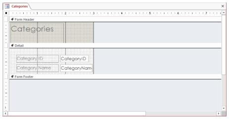
The design grid for the Categories form includes a Form Header that contains the title, a Details area that contains label and text box controls for two fields, and an empty Form Footer.
