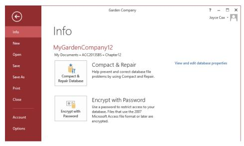
From this page, you can run utilities to help prevent database problems, assign a password, and assign file properties that help identify the file.
