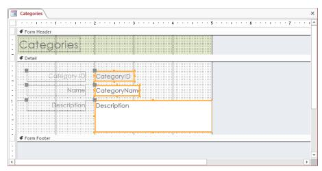
You have added a text box control and its associated label control, and changed the controls' alignment, size, and spacing.
