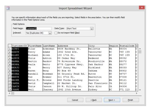
You can set the Data Type and Indexed properties of each field. You can also exclude a field from the import process.
